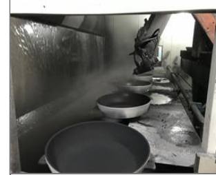
Photo of the inside of the main production hall 96 auto painting.JPG
